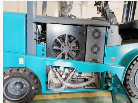
Solid-state hydrogen storage forklift and side-pull quick-swap technology
